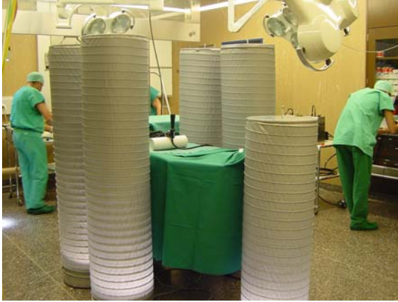
Figure 1a. An operating room at Zurich University Hospital shows heated person simulators that represent the surgeons.
